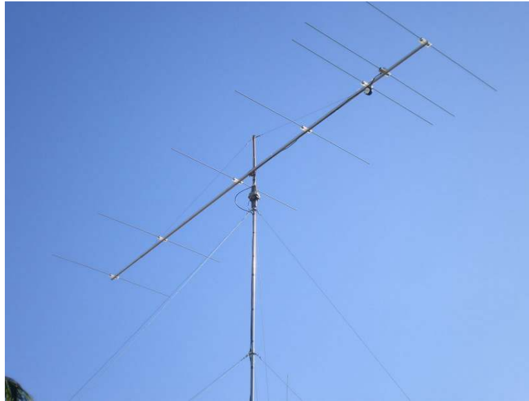
Wayne's VK4WTN 7 element YU7EF design yagi.
